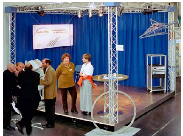
Flat turntable \varnothing 3.0 m, height 160 mm, load capacity 2000 kg, on our minimized booth on fair in 2003
