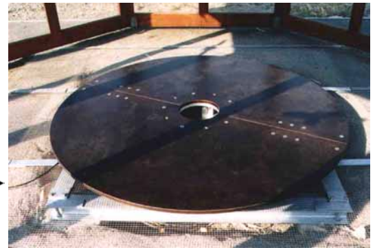
RST 070, this flat square module is mainly designed for installation into the false floor of a Fully-Anechoic Chamber, \varnothing 1.0 ... 1.5 m, load capacity up to 1000 kg, min. height 130 mm
