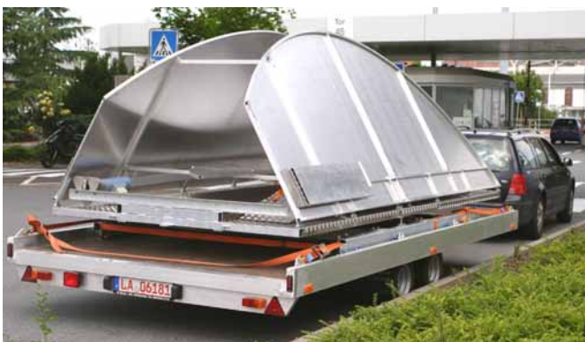
Designed for Adam Opel AG: Mobile turntable \varnothing 5.5 m including tilt-trailer, for the measurement of characteristics of car-antennas
