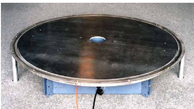
RST 040, for installation into the false floor of a Semi-Anechoic Chamber, \varnothing 1.0 ... 1.5 m, load capacity 400 kg, overall height c. 180 mm, also for OATS's
